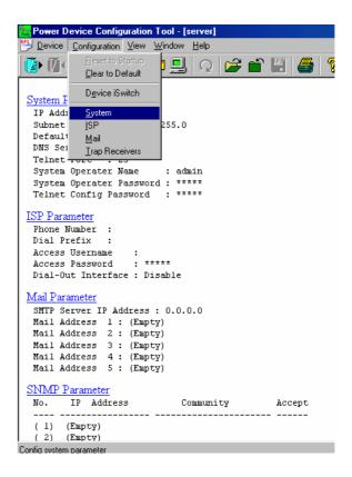
22. This is the System Parameter Configuration screen fill in all the information: the IP Address, the Subnet Mask, the Default Route (Gateway) and the DNS Server. Use the Tab key to move from one field to the next field. Then click OK.
